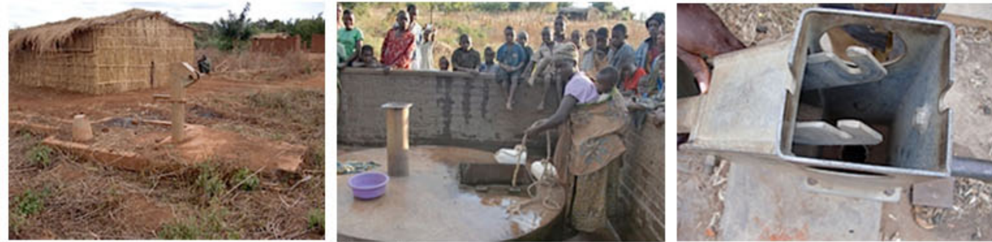
Photographs of broken VLOM water pumps. Taken by Water Works during a rural water point sustainability survey in Malawi, 2009.
